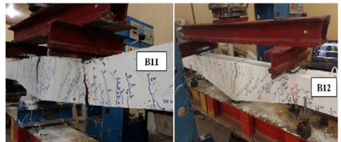
Fig. (24): Crack Pattern for B11
