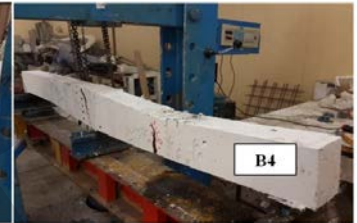
Fig. (14): Crack Pattern for B4
