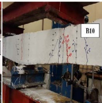
Fig. (22): Crack Pattern for B10
