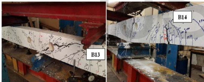
Fig. (27): Crack Pattern for B13
