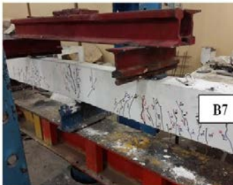
Fig. (17): Crack Pattern for B7
