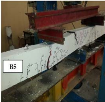
Fig. (15): Crack Pattern for B5
