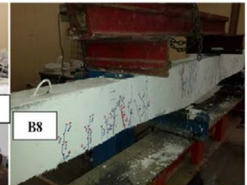
Fig. (18): Crack Pattern for B8
